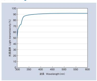
サンプル:100℃×1h+150℃×3h 試験片厚み:2mm Sample:Cured at 100℃×1h+150℃×3h Test strip thickness:2 mm
