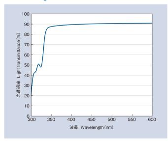
70℃×1h+150℃×5h硬化 厚み: 2 mm Cured at 70℃×1h+150℃×5h Thickness: 2 mm
