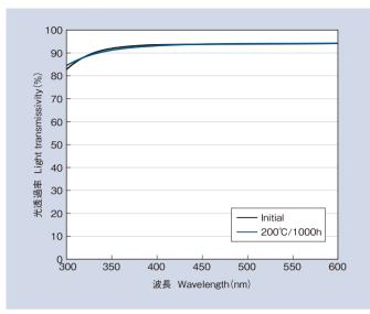
KER-2500: 100℃×1h+150℃×5h硬化 厚み: 2 mm Cured at 100℃×1h+150℃×5h Thickness: 2 mm
