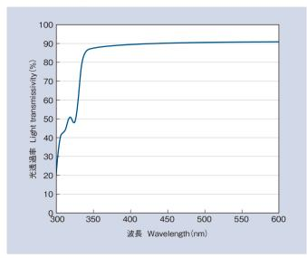
100℃×1h+150℃×5h硬化 厚み:2 mm Cured at 100℃×1h+150℃×5h Thickness:2 mm
