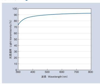
100℃×1h+150℃×3h 試験片厚み:2mm Cured at 100℃×1h+150℃×3h Test strip thickness:2 mm
