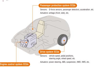
Sensors: temperature, pressure, flow rate, crank position, oxygen, NOx, water temperature, etc. Actuators: air flow, injectors, valve timing, etc.
