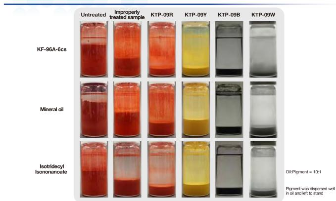
When pigments aggregate in oil, then precipitate, the precipitate becomes bulky, but the KTP-09 series is significantly less bulky in all three oils. This shows that these pigments have high wettability in a wide range of oils and inhibit aggregation.
