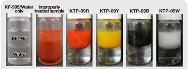
KF-995 (Cyclopentasiloxane): Water: Pigment=10g:10g:0.05g Pigments dispersed in KF-995, water added. Mixture shaken and left to stand, then observed.
