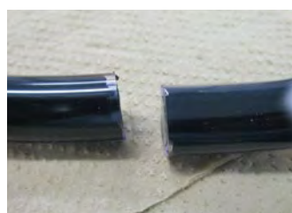
3-5 hours after potting Consistency: Rubber elastic body
