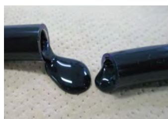
30 minutes after potting Consistency: Liquid
