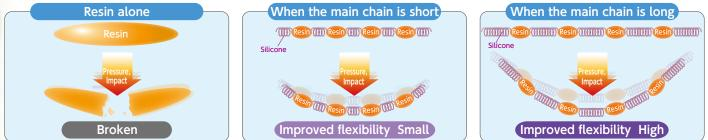
Model of water repellency and slip property improvement by graft copolymerization of single-end type
