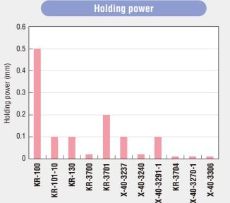
Substrate: stainless steel panel. Probe tack: contact pressure: 20 g/cm² probe speed: 1 cm/sec., contact time: 1 sec. Measured at room temperature (23-25°C).
