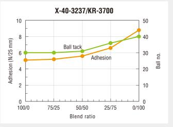
Backing: polyimide film, 25  $\mu m$  thick; PSA thickness 30  $\mu m$ Adhesion: Substrate: stainless steel panel. Ball tack: 30° slope. Probe tack: contact pressure: 20 g/cm², probe speed: 1 cm/sec., contact time: 1 sec. Measured at room temperature (23-25°C)
