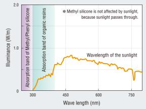
Much of the sunlight reaching the earth's surface is at wavelengths of 300 nm and higher. Most organic resins are susceptible to damage by light in this area of the spectrum. In contrast, Methyl silicone resins absorb almost no light in the UV spectrum, while Methyl/Phenyl silicone resins absorb only light in the spectrum below 280 nm, which means that sunlight has almost no effect.
