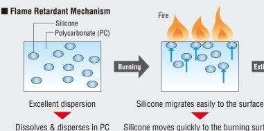
Silicone moves quickly to the burning surface
