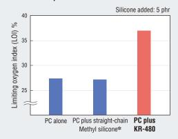
\* Weight-average molecular weight of silicone: around 60,000 (Data on PC resin provided by NEC Corp.)
