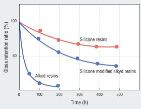
The graph above shows the gloss retention as tested by weatherometer. With an organic resin (alkyd), the drop is dramatic. But the silicone resin and silicone-modified alkyd resin retain much of their original luster.
