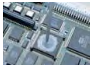
Thermal interface for CPUs
