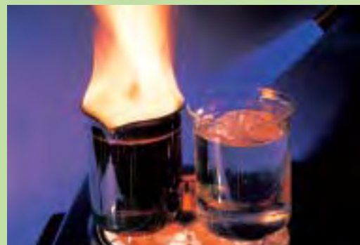
Heat resistance comparison (Left: mineral oil Right: silicone fluid)
