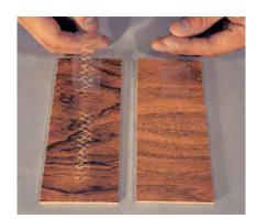
Separation test with cellophane tape on plywood (Left: Without silicone. Right: With silicone.)
