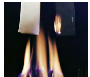
Flammability test Left: Silicone rubber Right: Organic rubber
