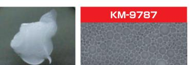
Coating synthetic leather with urethane resin containing 1 % silicone
