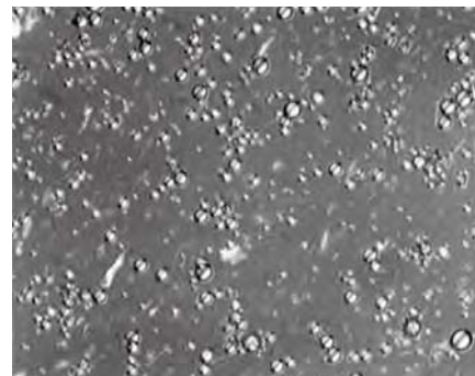
液状エポキシ樹脂への分散性(KMP-601) Dispersion toward fluid epoxy resin(KMP-601)
